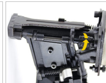
Adjusting the nailing depth by turning the inner crew
