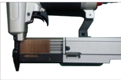
IF use mini brad the head should be upward.
